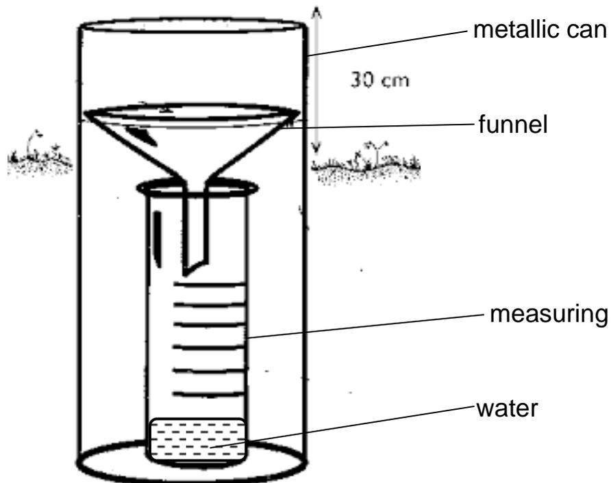
**A rain gauge** should be placed at least 15cm below the ground.
